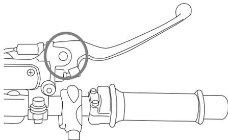
The operation of the brake and clutch levers should be checked before each ride, and the lever pivots should be lubricated if necessary.
