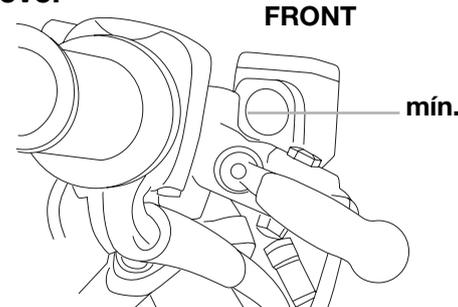
Insufficient brake fluid may allow air to enter the brake system, possibly causing it to become ineffective.
