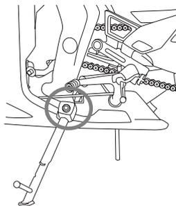
The operation of the sidestand should be checked before each ride, and the sidestand pivot and metal-to-metal contact surfaces should be lubricated if necessary.
