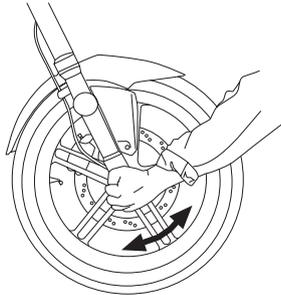
Worn or loose steering bearings may cause danger. Therefore, the operation of the steering must be checked as follows at the intervals specified in the periodic maintenance and lubrication chart.
