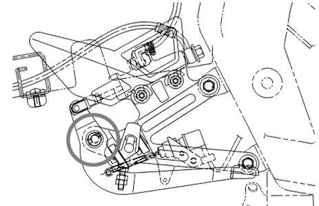
The operation of the brake and shift pedals should be checked before each ride, and the pedal pivots should be lubricated if necessary.
