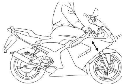
The condition and operation of the front fork must be checked as follows at the intervals specified in the periodic maintenance and lubrication chart.
