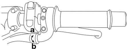
1. Loosen the locknut.
