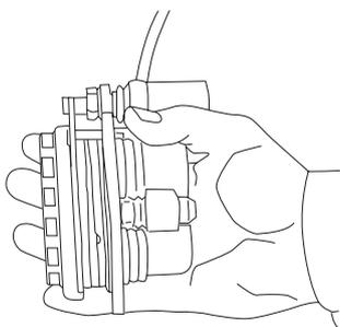
Each front brake pad is provided with a wear indicator groove, which allows you to check the brake pad wear without having to disassemble the brake. To check the brake pad wear, check the wear indicator groove. If a brake pad has worn to the point that the
