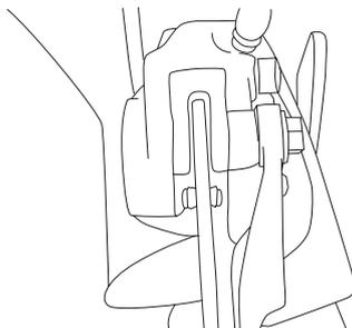
Each rear brake pad is provided with a wear indicator groove, which allows you to check the brake pad wear without having to disassemble the brake. Check the brake pad wear as follows.
