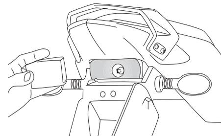
1. Remove the lens by removing the screws.
