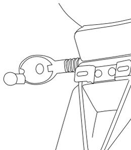
4. Install the lens by installing the screws.
