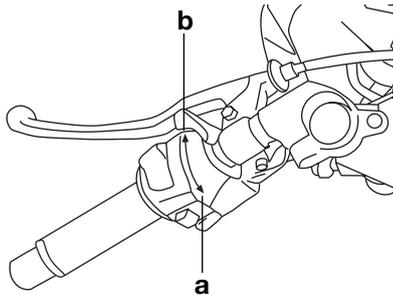
Starting a cold engine requires a richer air-fuel mixture, which is supplied by the starter (choke). Move the lever in direction (a) to turn on the starter (choke).
